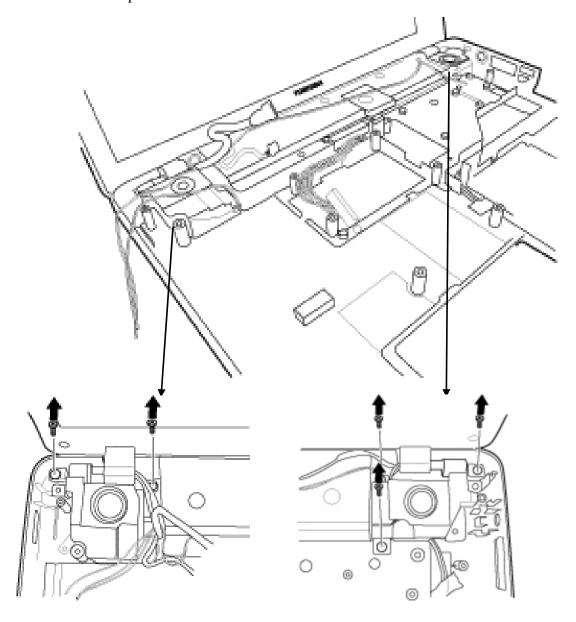
Figure 4-34 Removing screws securing speaker
